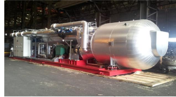
Pilot of Organic Rankine Cycle Waste Heat Recovery System for Steel Rolling Mill Reheating Furnace in Singapore
